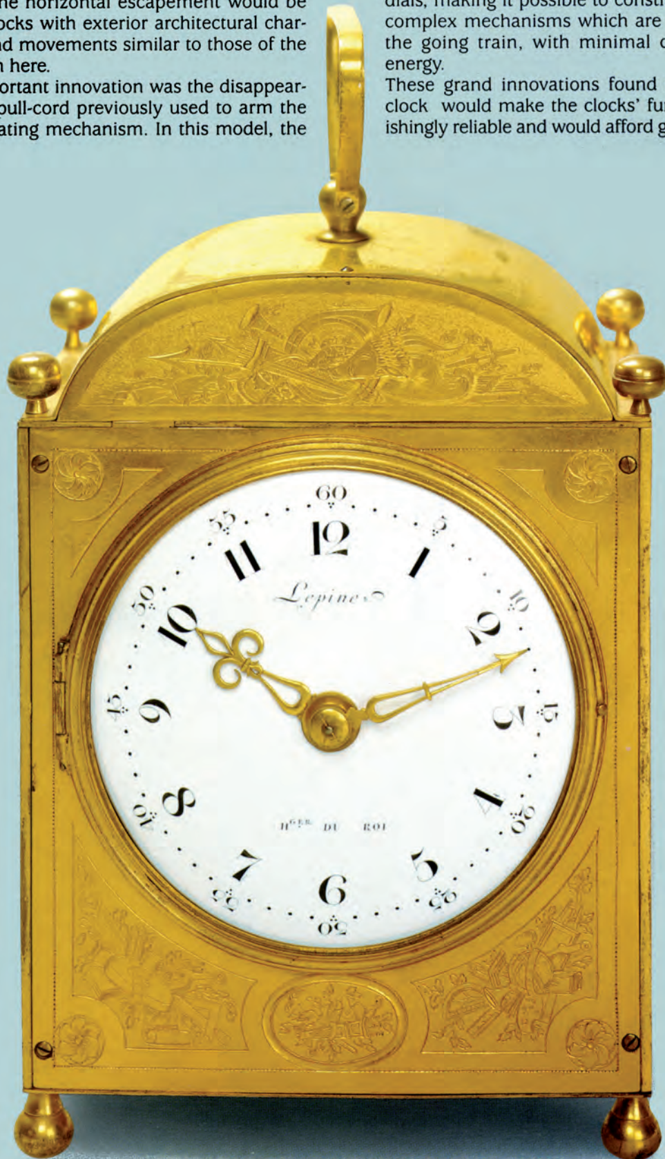
Lépine, Horloger du Roi à Paris, No. 4085, circa 1788. Eight day-going gilt brass carriage clock with hour and quarter striking, virgule escapement, and vertical balance and cock in the back plate. Height 21 cm.
